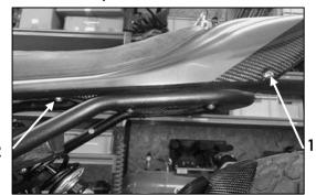
To re-fit seat, align the stud to the sub-frame (2) and press down the carbon tail unit onto the sub-frame. Replace all the fixings.
