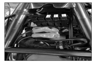
To remove the tank, first remove the seat, remove the 2 bolts (1) and slide the tank backwards. Making sure to disconnect the fuel line and the fuel pump connector.
