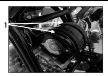
To access the battery, removal of the battery cover is required. To remove the cover, remove the straps (1) then slide the cover rearwards and away from the battery.
