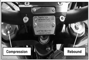
The compression and rebound can be adjusted by turning the middle adjuster with a flat screwdriver.
