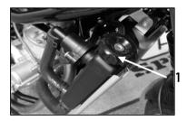
Coolant minimum level is defined by the internal top plate. Maximum level is
