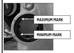
Ensure the oil level is between the maximum and minimum marks on the lefthand side of the oil level inspection window.
