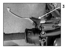
When starting the engine with a cold engine pull the cold start lever (3), keep the lever depressed until the engine temperature is warm enough to tick over.
