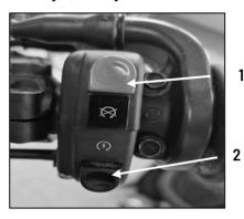
To turn the engine off, press and hold the "KILL" button (1).
