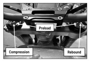
The Ohlins front forks adjust in the same way as the Marzocchi forks, a 2.5mm Allen key is used to adjust the compression and rebound & a 14mm spanner is used to adjust the pre
