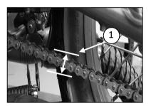
To adjust chain slack, loosen the rear wheel nut and use the chain adjuster bolts to achieve recommended chain slack. Check the wheel alignment, re-tighten adjuster bolts, adjuster lock nuts and rear wheel nut.
