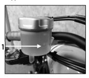
Check the fluid level in the rear master cylinder is above the minimum marker (1)
