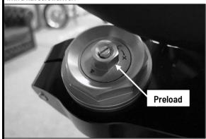
The front fork preload can be adjusted by turning the outer 14mm flange on the top of the fork with a 14mm spanner.
