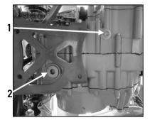
Remove the oil sump plugs (1&2) and allow oil to drain into drain pan.
