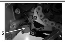
Once most of the oil is drained remove the oil strainer (3) by unscrewing the 2 fastening bolts and inspect for debris, clean and replace.
