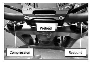
The Ohlins front forks adjust in the same way as the Marzocchi forks, a 2.5mm Allen key is used to adjust the compression and rebound & a 14mm spanner is used to adjust the pre
