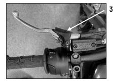
When starting the engine with a cold engine pull the cold start lever (3), keep the lever depressed until the engine temperature is warm enough to tick over.
