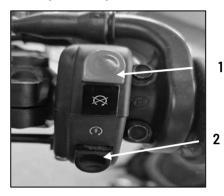
To turn the engine off, press and hold the "KILL" button (1).
