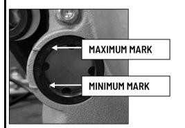
Ensure the oil level is between the maximum and minimum marks on the lefthand side of the oil level inspection window.
