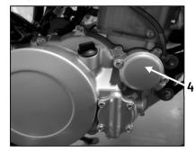
Remove the oil filter cover (4) and oil filter element.
