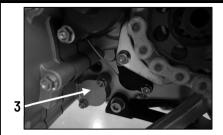
Once most of the oil is drained remove the oil strainer (3) by unscrewing the 2 fastening bolts and inspect for debris, clean and replace.
