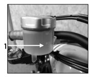
Check the fluid level in the rear master cylinder is above the minimum marker (1)
