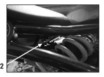
To re-fit seat, align the bosses of the bottom of the tail piece, the stud to the sub-frame and replace the fixings.
