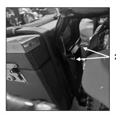
Using a 5mm Allen Key & 13mm spanner remove the 2x Nut (2) & Bolts (1)
